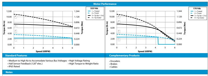
$1. Test\ conditions: Motor\ operated\ at\ rated\ winding\ temperature,\ mounted\ to\ an\ aluminum\ heat-sink.$
